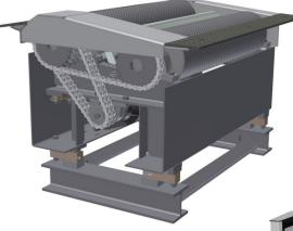
As standard, the **rear rollers** on the RT9241 are **raised** and each pit is equipped with it's own integrated electronic box including star-delta switching. A seperate relay box is not required. Also standard are the electronic motor brake, automatic slip detection and mains power box containing main switch, emergency stop, ON/OFF light indicator.
